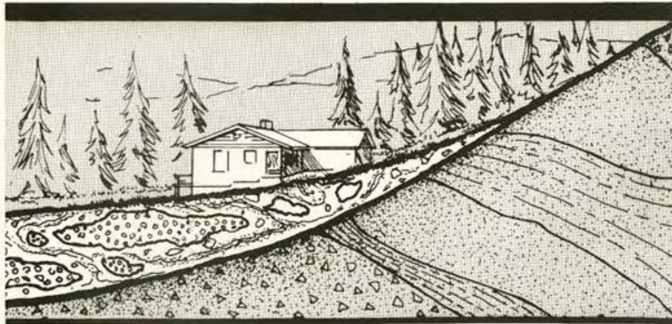
Differential settlement can be expected (as a result of variable distribution and thickness of alluvium) in response to normal consolidation, imposed static load, and seismic shock.
